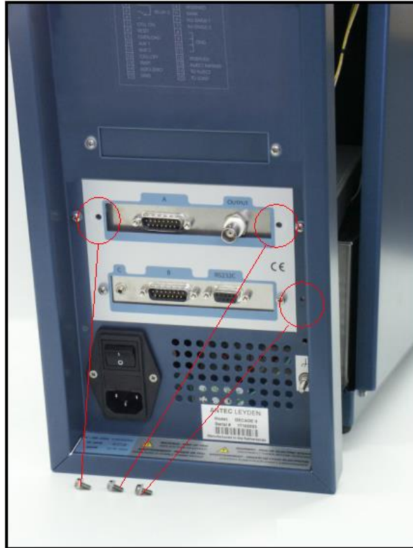
Fig. 7. Removal of sensor board from the connector panel.
