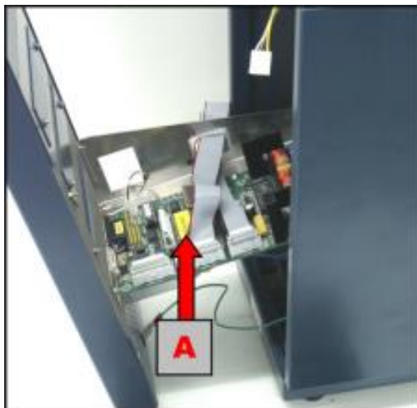
Fig. 7. Removal of sensor board from the connector panel.
