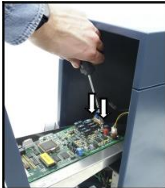
Fig. 6. Removal of internal cell cable connector.
